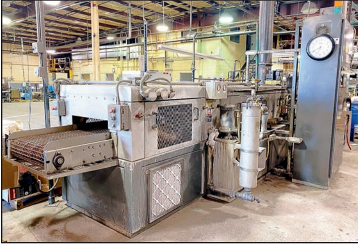
HURRICANE SYSTEMS 5024 PRE-WASH/WASH/RINSE/BLOW-OFF LINE
