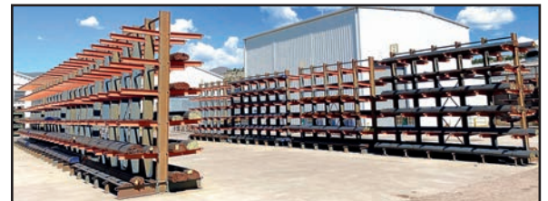
VIEW OF BAR STOCK AND CANTILEVER RACKING
