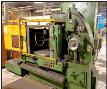
BLANCHARD NO. 18-42 ROTARY SURFACE GRINDER
