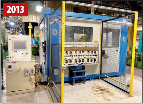
ACT RFC-50.2-T ROBOTIC FINISHING CELL
