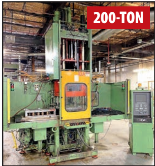
ENGEL ES600/200VSH VERTICAL INJECTION MOLDER
