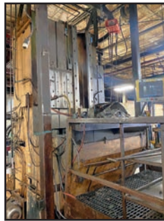
DETROIT BROACH VTT-15-66 15-TON X 66" DOUBLE RAM VERTICAL BROACH
