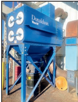
DONALDSON TORIT DOWNFLO EVOLUTION DFE2-8 DUST COLLECTOR
