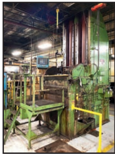
LAPOINTE 15-TON X 66" DOUBLE RAM VERTICAL BROACH
