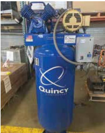
QUINCY QT55QCB AIR COMPRESSOR
