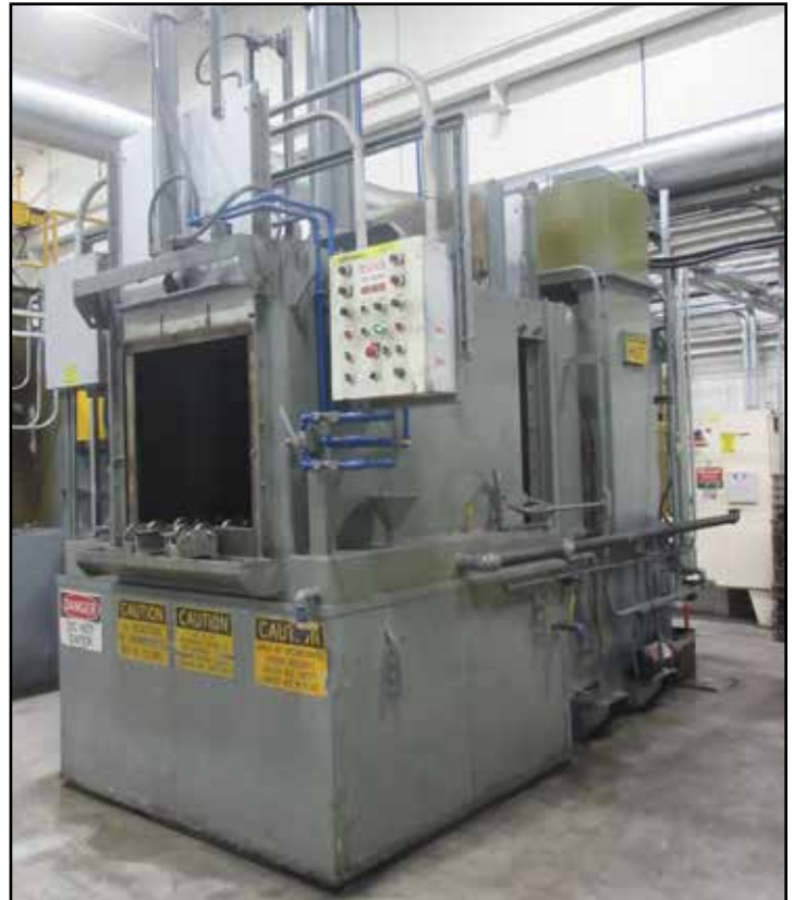
SURFACE COMBUSTION WILLIAMS PRE/POST CARBURIZING 2 STAGE WASH SYSTEM
