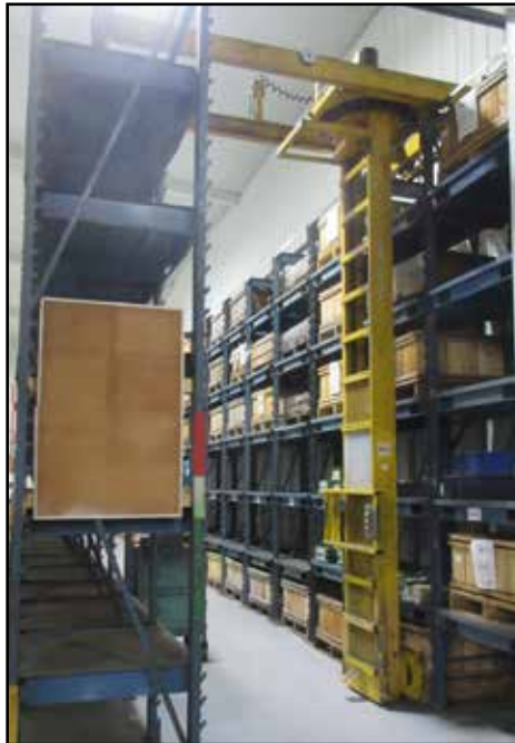
2,000 LB STORAGE/RETRIEVAL CRANE & RACKING SYSTEM
