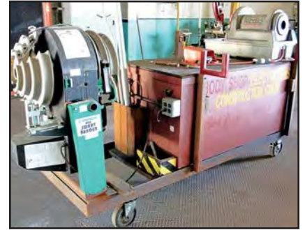
GREENLEE 855 SMART BEND W/RIDGID 300 PIPE THREADER
