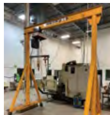
HANDLING SYSTEMS 3-TON ROLLING GANTRY
