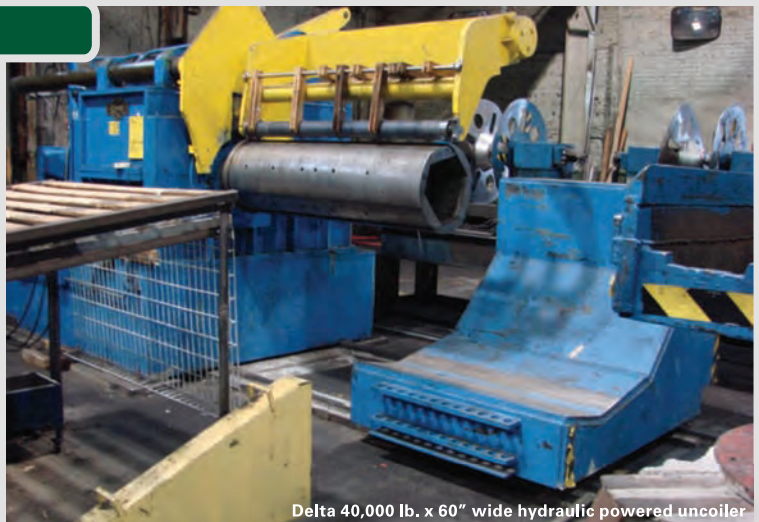
Delta 40,000 lb. x 60" wide hydraulic powered uncoiler
