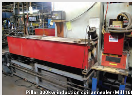
Pillar 300kw induction coil annealer (Mill 16)
