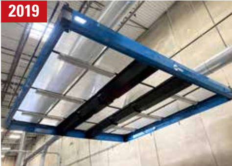
MILLER FILTAIR 6000 WELDING FUME EXTRACTION SYSTEM
