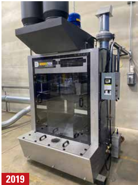
DIVERSITECH TYPHOON WX-6500 WET TYPE DUST COLLECTOR
