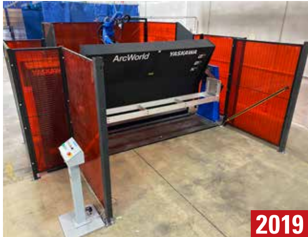
YASKAWA MOTOMAN ROBOTIC WELDING CELL & POSITIONER
