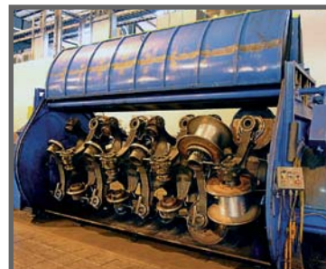
KRUPP 24-BOBBIN SECTION ON THE 54-WIRE STRANDER
