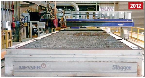
MESSER MPC2016 (3)-HEAD CNC PLASMA CUTTING SYSTEM
