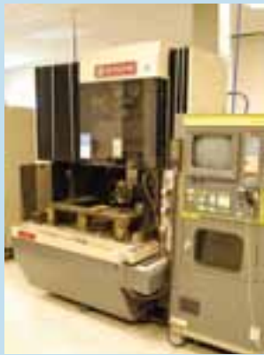
Hitachi 460QAWF CNC Wire Electrical Discharge Machine, S/N: D410249005 (1989); X Travel-26", Y Travel-18", Z Travel-12", Die Electric Coolant Filtration, Oilmatic KTV-3B-C1 Chiller, Fanuc HP CNC/CRT Control
