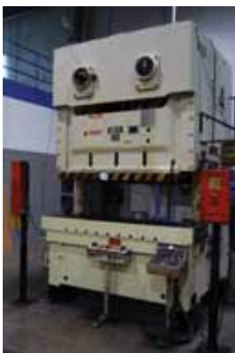
176 Ton Aida NC2-160 Double Crank Gap Frame Mechanical Press, S/N: 10516-1123; 80" x 23.6" Bed Size, 5.11" Stroke, 3.9" Adjustment, 15.9" Die Height, 40-85 SPM, Clarkton Digital Tonnage Monitor, Link-Lite Safety Curtains
