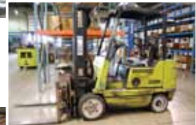
7,000 LB Clark CH70 LP Gas Forklift, S/N: 77-702; 153" Lift, Triple Mast, Hard Tires
