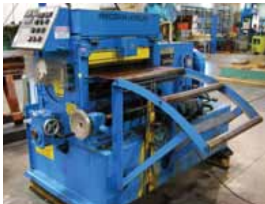
Herr-Voss VML025/1.50-17/3 LH Mini Leveler, S/N: 41986-001 (1994); .080" x 24" Width Capacity, LH Mini Leveler, Control Panel with LED Display
