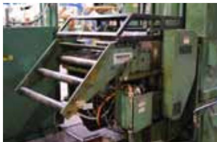
Minster Feed Line Comprising: Minster MEF6-26 Servo Feed, S/N: 1850266; .312" x 26" Wide Capacity Minster 30-26-7 Straightener, S/N: 13-50133; .312" x 26" Wide Capacity, 7 Over 8 Roll Configuration, Peeler Blade Control Panel with LED Display.
