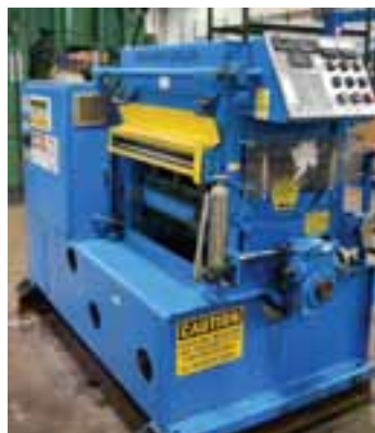
Herr-Voss VML025/1.50-17/3 LH Mini Leveler, S/N: 41986-001 (1994); .080" x 24" Width Capacity, LH Mini Leveler, Control Panel with LED Display
