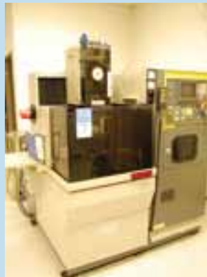
Hitachi H-Cut 203 CNC Wire Type Electrical Discharge Machine, S/N: D310388005 (1988); X Travel-18", Y Travel-12", Z Travel-12", Die Coolant Filtration System, Fanuc HF CNC/CRT Control
