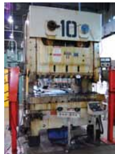
121 Ton Aida NC2-110 Double Crank Gap Frame Mechanical Press, S/N:10511-1055; 74" x 20.4" Bed Size, 4.33" Stroke, 3.5" Adjustment, 13.7" Shut Height, 20-100 SPM, Imco Tonnage Monitor, Link-Lite Safety Curtain
