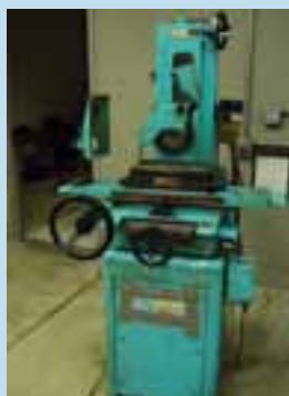
6" x 12" Boyer Schultz H612 Hand Feed Horizontal Surface Grinder, S/N: 227486 (1976); Walker 6" x 12" Fineline Electromagnetic Chuck & Electromagnetic Chuck Control
