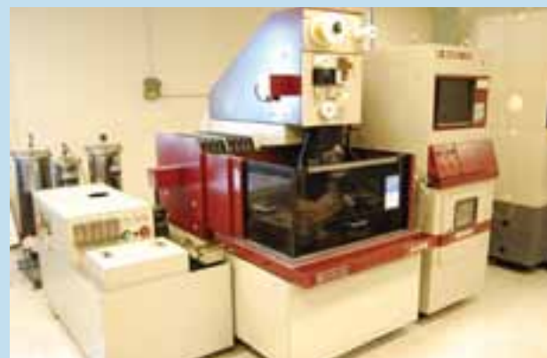
Hitachi Model 235Q CNC Wire Type Electrical Discharge Machine, S/N: D310991002 (1991); X Travel-22", Y Travel-16", Z Travel-14" Die Electric Coolant Filtration, H-Mark-100 CNC/CRT Control & Remote Pendant
