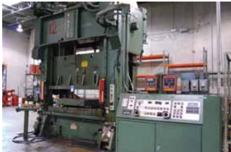
300 Ton Minster E2-300-96-48 HEVISTAMPER Straight Side Double Crank Mechanical Press, S/N: 27641 (1990); 96" x 48" Bed Size, 8" Stroke, 6" Adjustment, 30" Shut Height, 0-100 SPM, 28" x 15" Windows, Minster Programmable Control, Wintriss Diepro 1500 Die Protection & Wintriss Autoset 1500 Load Analyzer
