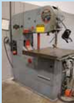
Doall 3613-1 Vertical Bandsaw, S/N: 440-90387 (1990); 36" Capacity; 50-5200 SFPM Blade Speed, 30" x 30" Table
