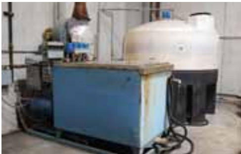
Samso 75,000 BTU 700-316 Water Evaporator, S/N: 01184; Power Flame Gas Burner, 25-HP Exhaust Fan, Stainless Steel Coolant Tank, Cutler Hammer Programmable Temperature Controls, Omron Digital Timer
