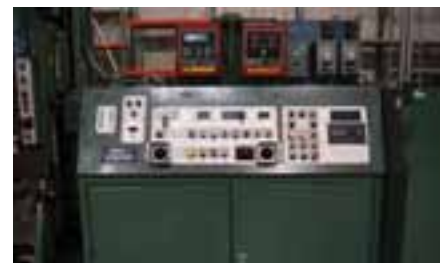
Minster Feed Line Comprising: Minster MEF6-26 Servo Feed, S/N: 1850266; .312" x 26" Wide Capacity Minster 30-26-7 Straightener, S/N: 13-50133; .312" x 26" Wide Capacity, 7 Over 8 Roll Configuration, Peeler Blade Control Panel with LED Display.
