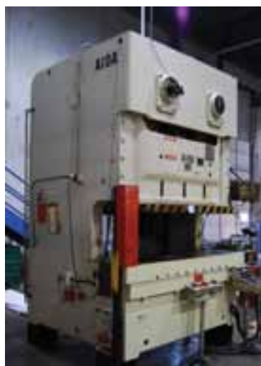
176 Ton Aida NC2-160 Double Crank Gap Frame Mechanical Press, S/N: 10516-1123; 80" x 23.6" Bed Size, 5.11" Stroke, 3.9" Adjustment, 15.9" Die Height, 40-85 SPM, Clarkton Digital Tonnage Monitor, Link-Lite Safety Curtains
