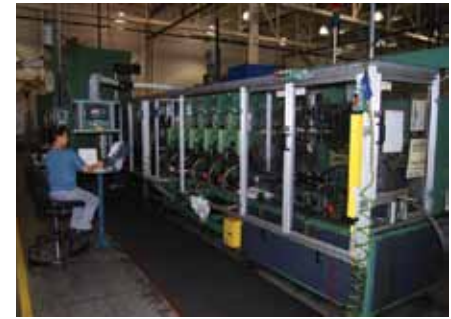
JEWETT AUTOMATION Terminal Connector Assembly Line
