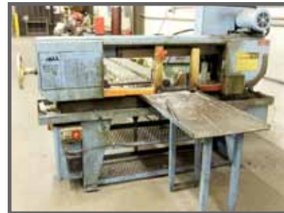
DOALL C-916 HORIZONTAL BANDSAW
