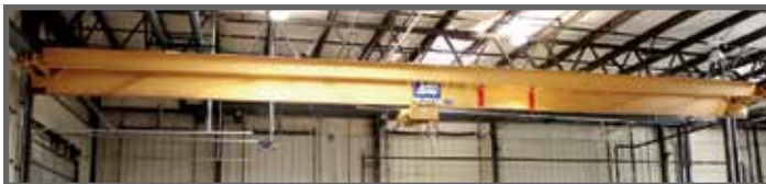
5 TON ACCO OVERHEAD CRANE
