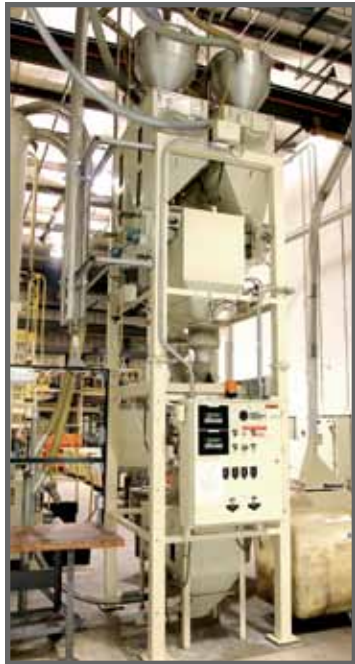
PACIFIC ENGINEERING (2) SCALES (4) HOPPERS DELIVERY SYSTEM
