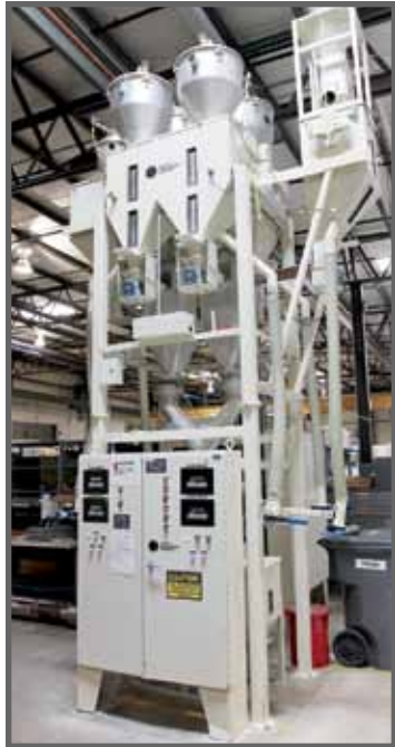
PACIFIC ENGINEERING (2) SCALES (6) HOPPERS DELIVERY SYSTEM
