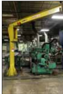
1 Ton GAFFEY Jib Crane with Jet Trolley
