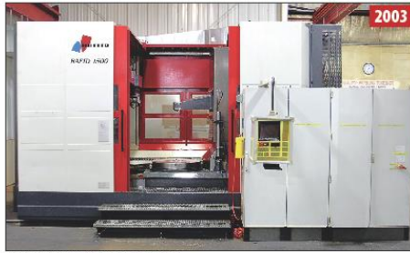
HOFLER RAPID 1500 7-AXIS CNC PROFILE GEAR GRINDER
