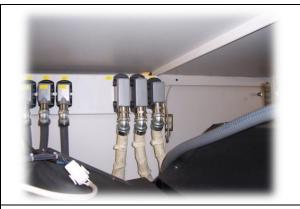
4. If equipped with nitrogen lines, disconnect these next.
