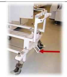
14. To install the new cart and solder pot, reverse the procedure. Verify rollout tracks are lined up, solder cart latching mechanisms are fully engaged, and rear wheels are locked before reversing this procedure.
