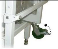
13. Push the locking release arm to unlock the cart from the machine and pull back on the cart. The cart is now free to move to its storage location.
