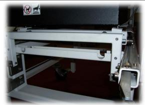
11. Secure the front toggle clamps on each side of the pot to the holes in the brackets that mount to the solder pot legs.
