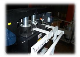
10. Raise the front trolley stop bracket and secure it in the up and locked position.
