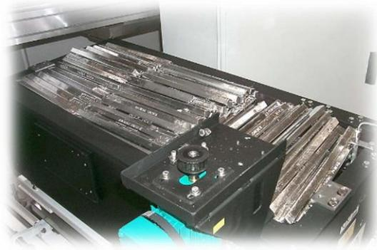
7. If equipped, load the solder bar feeder with bars as shown.
