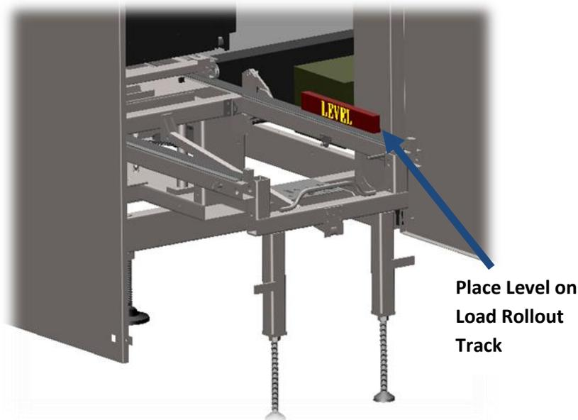
14. Adjust the load rollout stand leg until the level indicates proper positioning.
