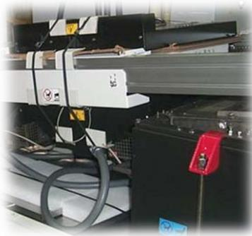
10. Remove the three (3) shipping brackets at the back of the solder pot.
