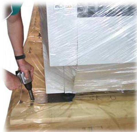
2. When all jam nuts are removed from the shipping plates, carefully position a fork lift, with the fork extensions at their widest setting, under the frame. Make sure that the forks make proper contact with the base beams to avoid damage to the wiring and metal panels underneath the machine.
