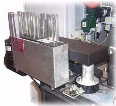
8. It is recommended that the solder pot be covered with a high temperature blanket during heat-up to minimize the solder eruption hazard. Consult the factory to obtain a blanket if not purchased with the machine.
