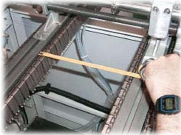
2. If the distances measured at all three (3) locations are within 1.5 mm (0.06 in.) the conveyor is within tolerance. If it is outside this tolerance contact the factory for instructions before making any adjustments.
