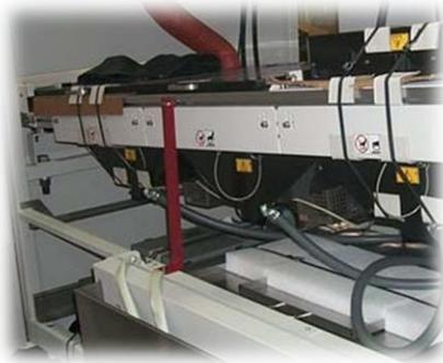
9. Remove the shipping bracket on the front of the solder pot.
