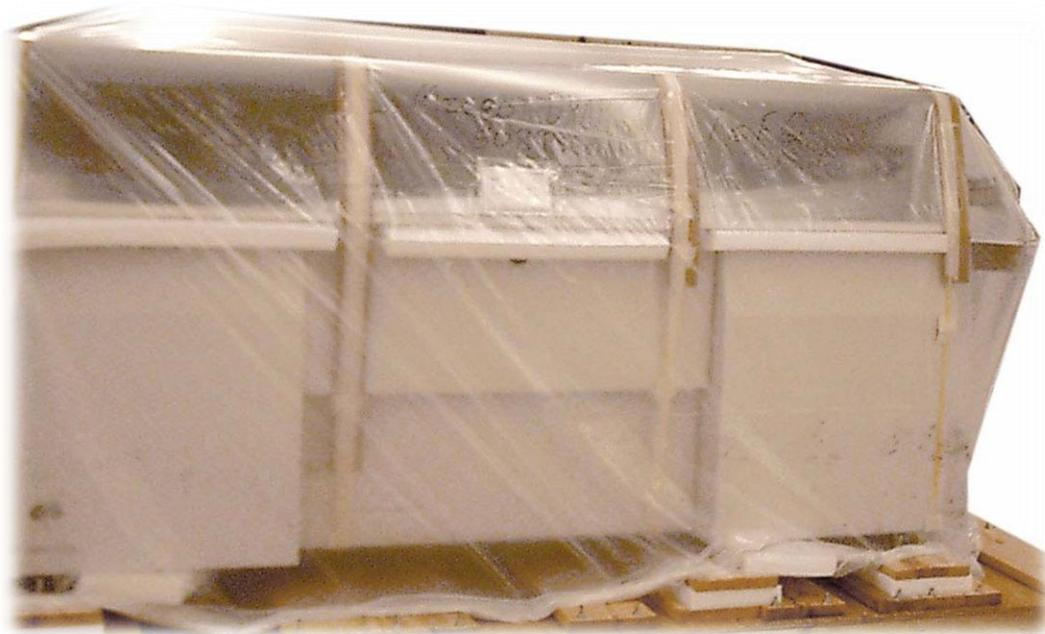
1. Remove the plastic wrapping from the perimeter of the system.
