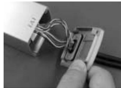
10. Affix the motor-end cap with the pan-head screws (M3 x 80, 4 pcs). At this time, pay attention not to pinch the cables.
