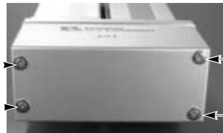
5. Hook a looped strong string (or long tie-band) on the motor bracket, pull the string with a tension gauge to the specified tension, and then securely and uniformly tighten the adjustment bolts (View B above).
