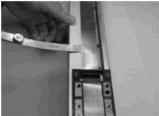
Tightening torque (SA6/SA7):Thin-head screw M3 x 6-87.2 N-cm (8.90 kgf-cm)
