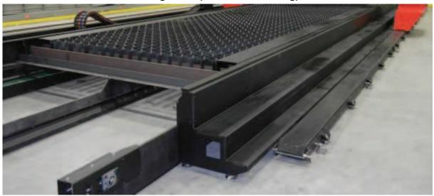
This design is the premier dry cutting table from Kinetic and is designed to be a safe and easy platform with support for 8" thick plates to be cut.
