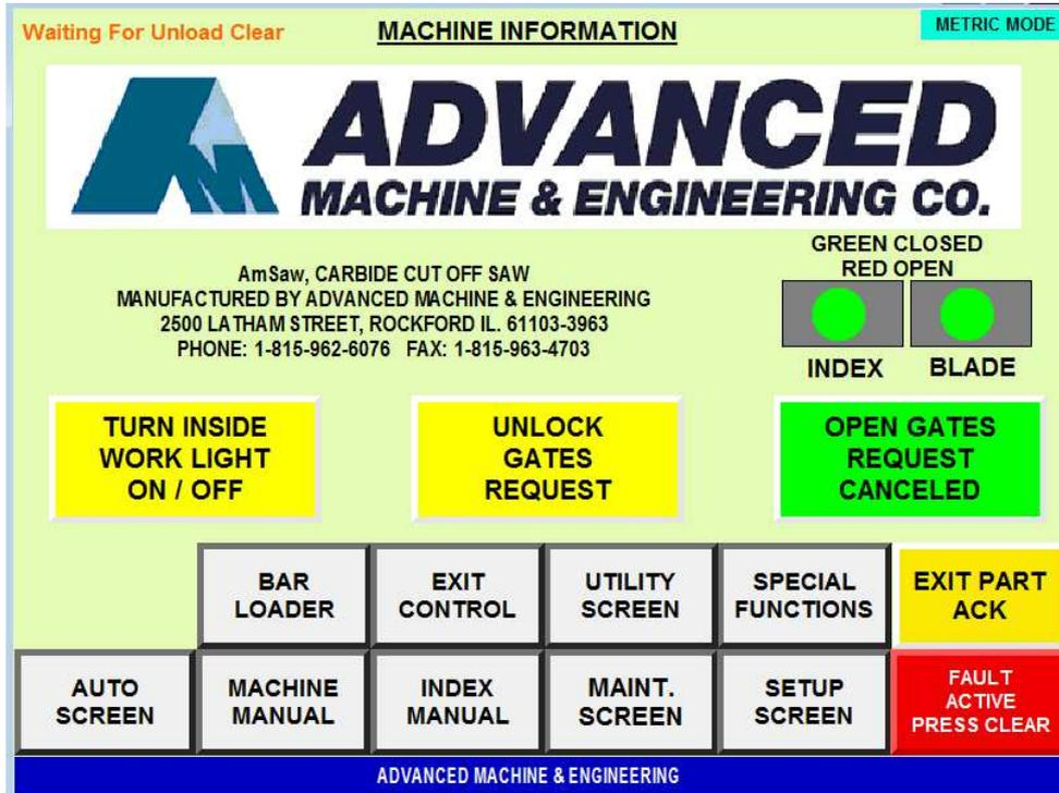
The Information and Gate / Light control screen is the default screen loaded when electric power is first applied to the machine...
