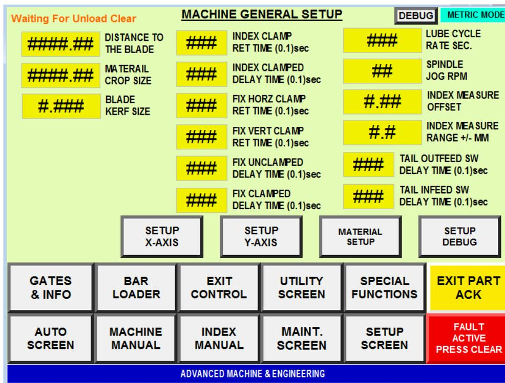
This screen Displays/Configures the General Machine Setup Data.
