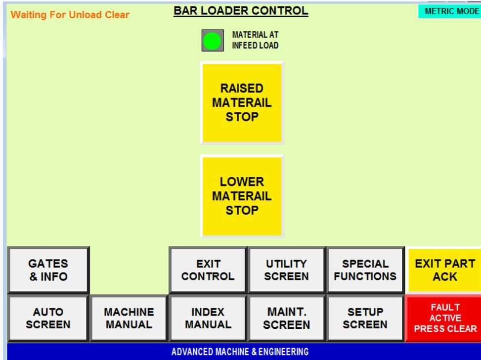
This screen is used for manually controlling the machine load function.
