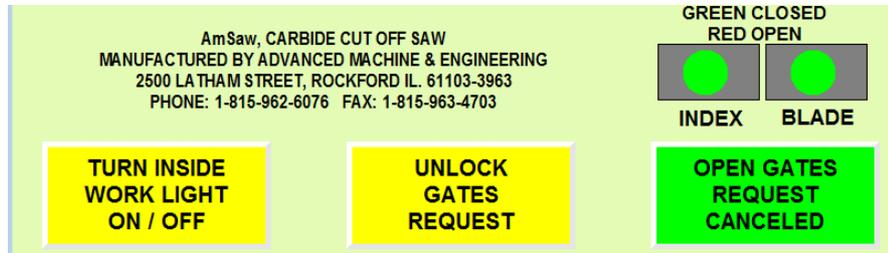
The gate locks are controlled by an internal solenoid in the gate switch that requires it to be energized to open.
