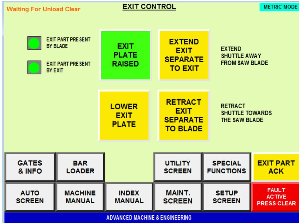
This screen Controls the Manual Movements of the Machine Exit System. .
