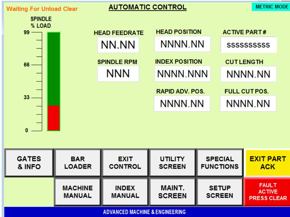
This screen is used to display the machine status.
