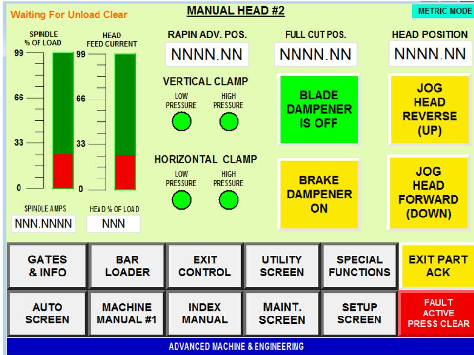
This screen is used to display spindle status, X & Y- axes status and Head Slide (X-Axis) Jog Commands.
