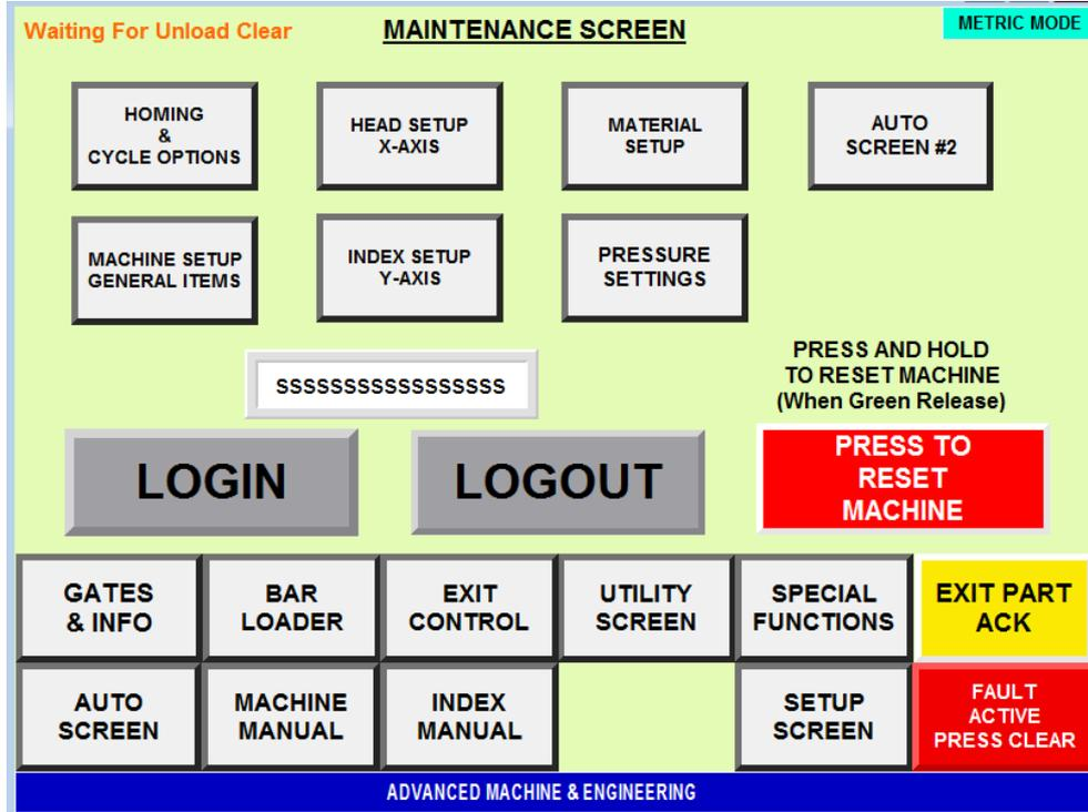
This screen is used to access the machine setup conditions. Items on the screen are password protected. This screen is also used to perform a machine Master Reset.
