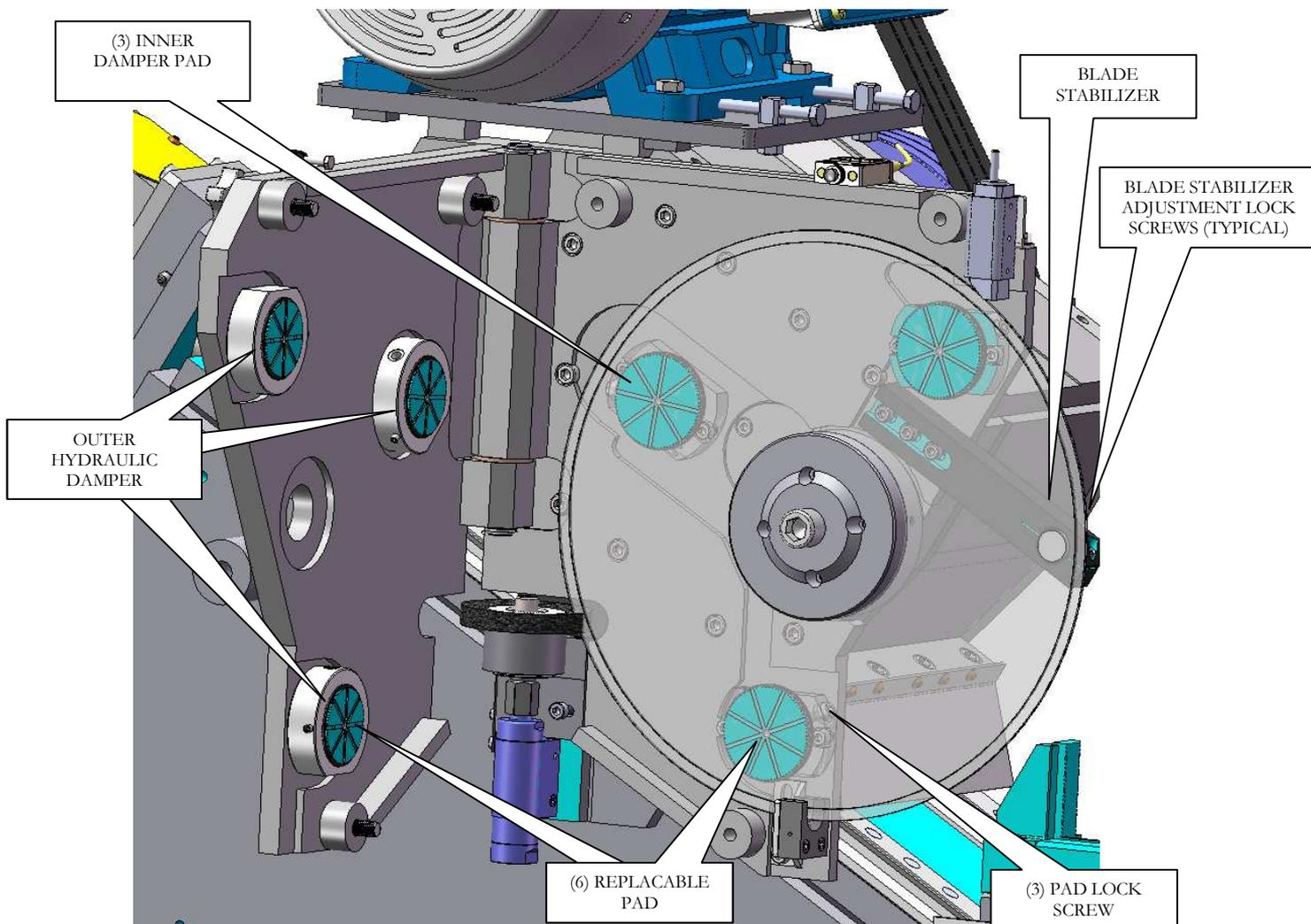
The three adjustable blade damper pads have been set-up to be in the same plane with the blade hub contact surface using a ground gauge bar. These pads are designed for long life and incorporate a locking mechanism in the mounting bracket. These features are incorporated so that the adjustment of the inner brake is not necessary.
