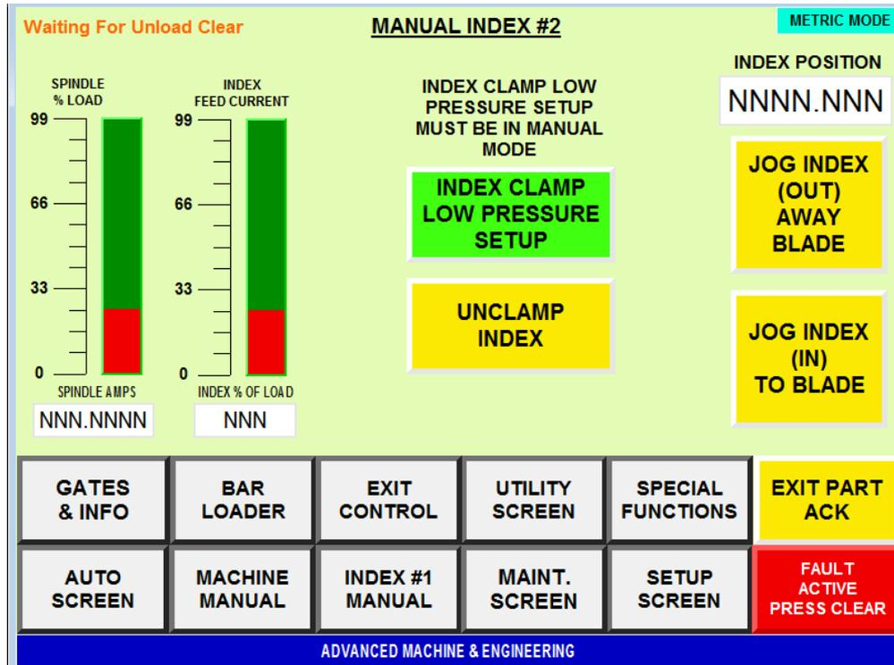
This screen is used to control the manual functions of the Index Slide and Index Clamp.
