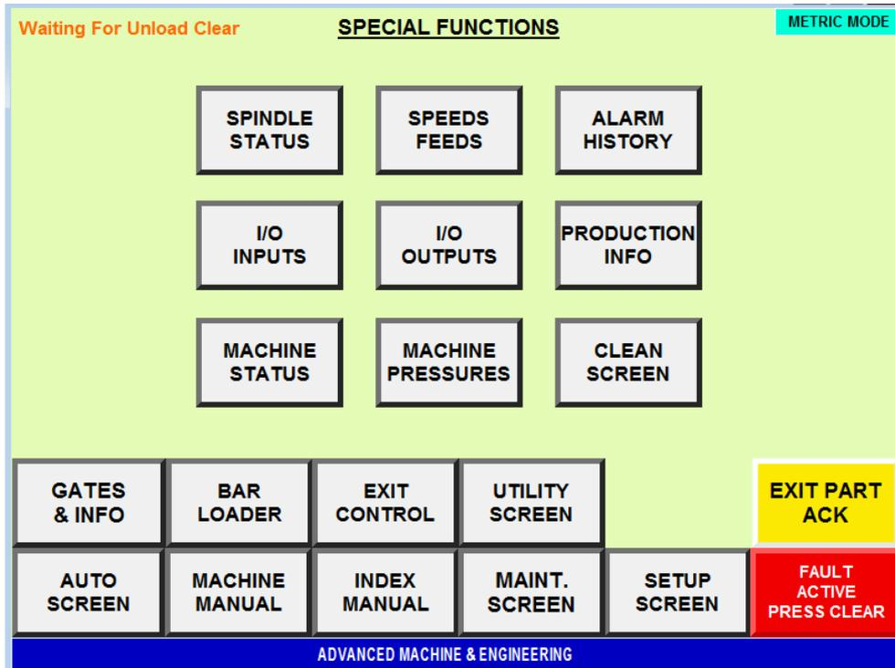
This screen is used to access additional machine special function screens.
