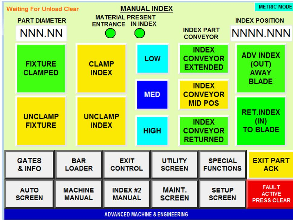
This screen is used for manual control of the index, Index Clamp and Fixture Clamps.
