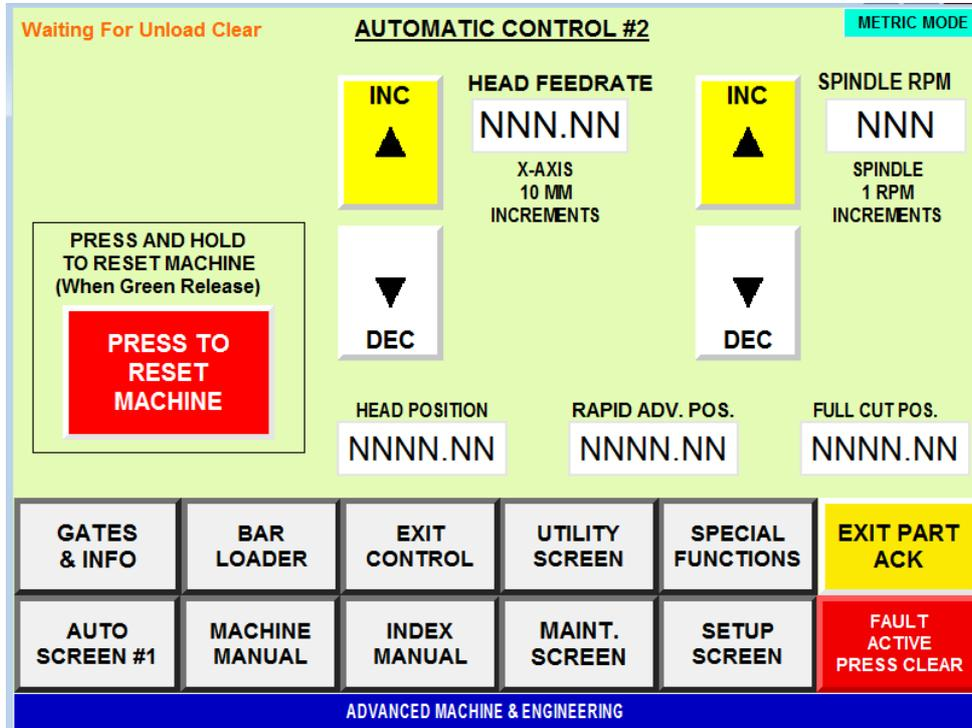
This screen is used to monitor and adjust spindle speed and Head Feed in Auto Mode. It is also where you could perform a Master Machine Reset.
