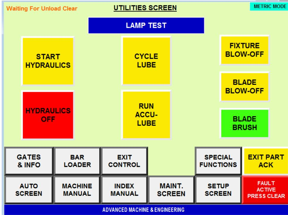
This screen is used for manual control of machine functions, Hydraulics on/off, Cycle Lube, Run Accu-Lube, Fixture Blow-off, Blade Blow-off and Blade Brush..
