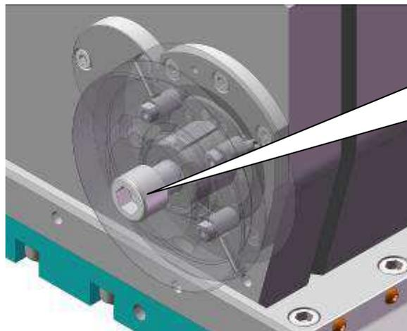
(1) Bolt M20 holding the Drive Hub to the spindle. In case of replacing or maintenance, the M20 bolt must be torque to 180 Ft-Lbs
