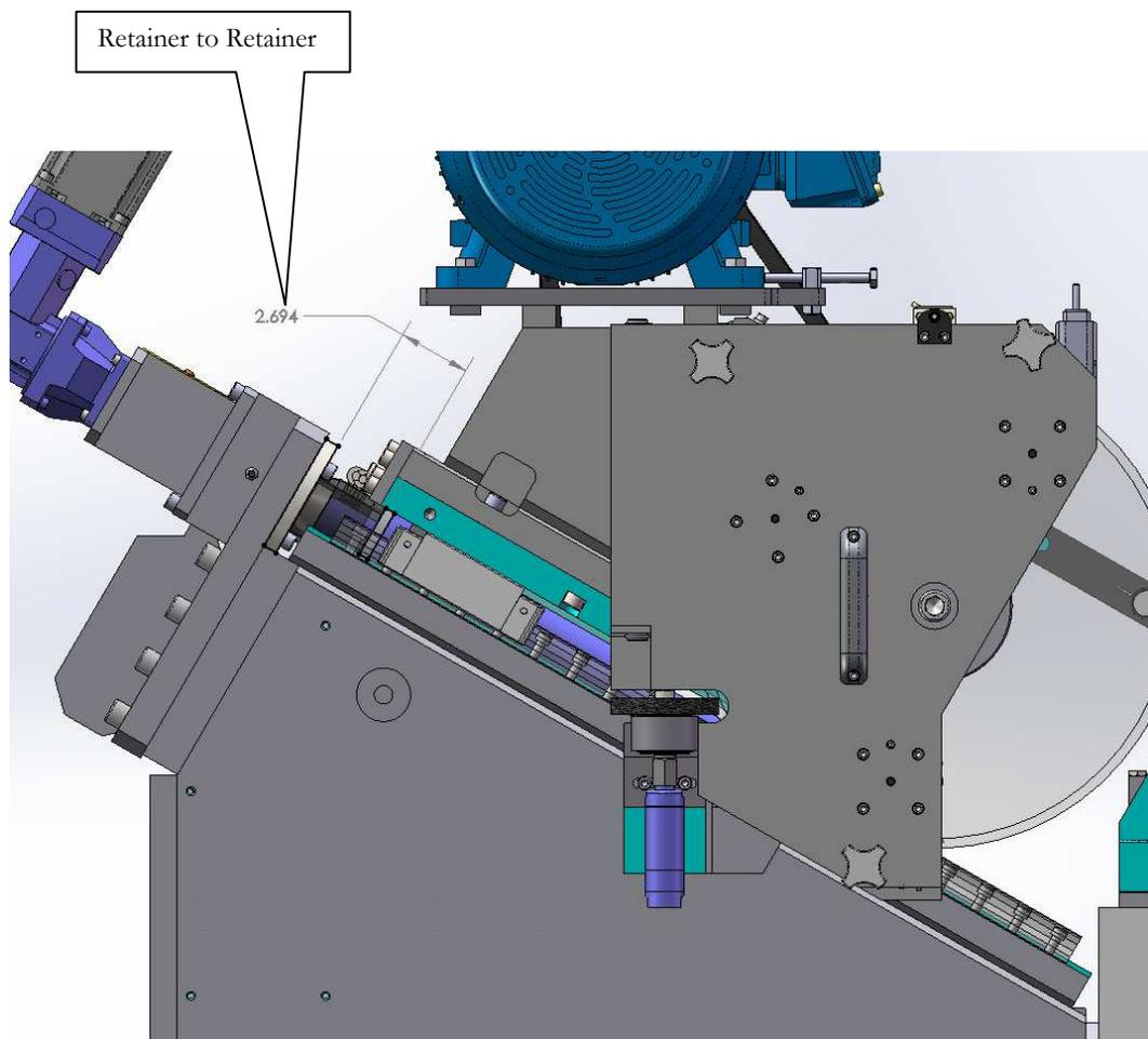
Measure the distance from “retainer to retainer” of the head feed ball screw. Manually jog the Head feed to the dimensions listed below to set the "home position".
