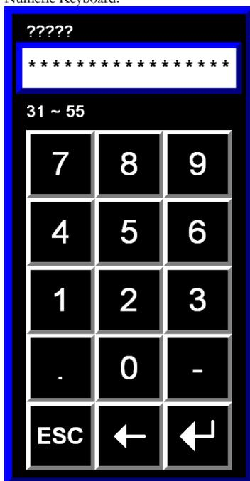
A Pop-up window is displayed when a data entry field (input field) is selected from any of the screens. Data entry fields contain a beige background color (e.g. Part Length, Blade Size, Material Size).
