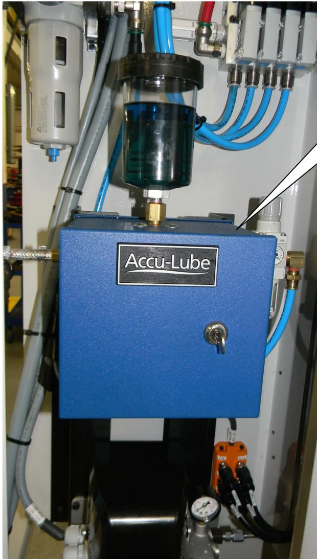
Accu-Lube Located on the Rear of the Base
