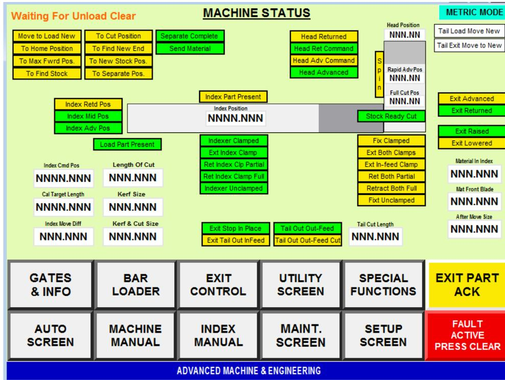
This screen is used to display the machine running status.
