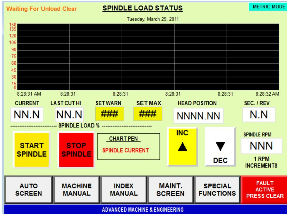
This screen is used to display and configure spindle load % information.
