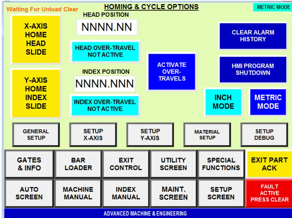
This screen is used for homing the X & Y Axes, Head and Index Positions
