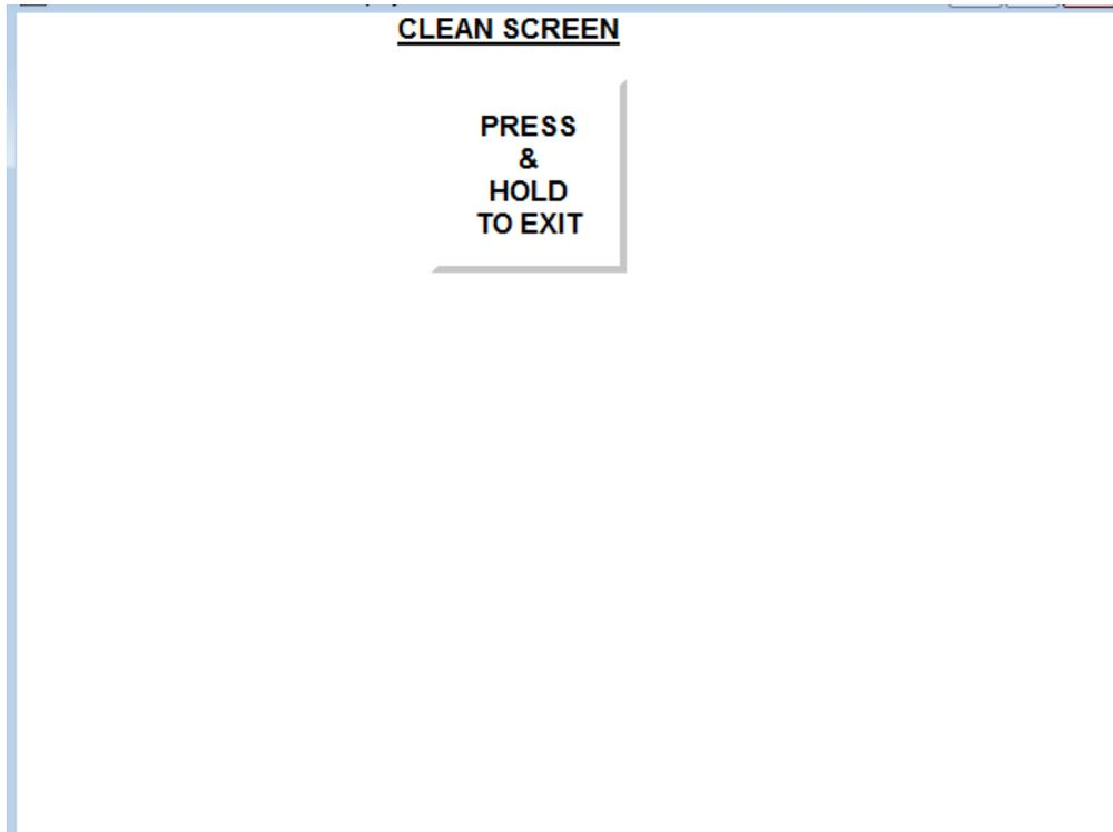
This screen is used to clean the HMI screen, without activating any commands.
