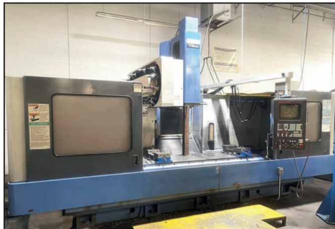
MAZAK MAZATECH MTV655/80 VERTICAL MACHINING CENTER
