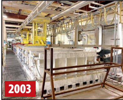
CLEARCLAD 26-STATION E-COAT LINE
