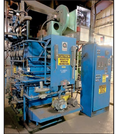
ATMOSPHERE FURNACE CO. 3000CFH ENDOTHERMIC GAS GENERATOR
