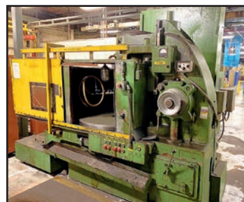
BLANCHARD NO. 18-42 ROTARY SURFACE GRINDER
