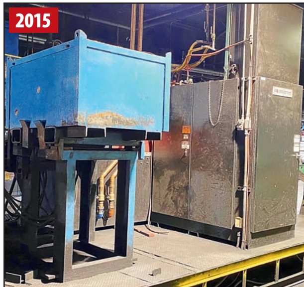
ESC INDUCTION IGBT800-1-3 800 KW INDUCTION HEATING SYSTEM
