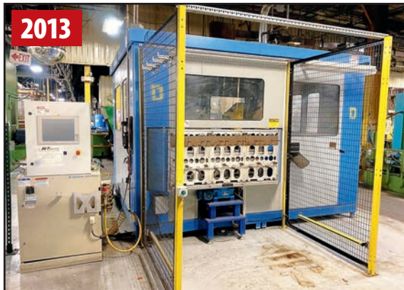
ACT FRC-50.2-T ROBOTIC FINISHING CELL
