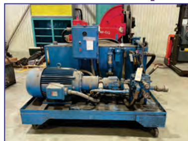
Tex-A-Draulics large, high volume hydraulic pump, with a 60 hp Toshiba induction motor
