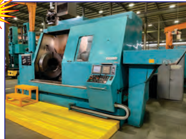
Warner & Swasey SC-32 CNC Chucker Lathe, 40" 3-jaw Big Bore chuck w/ 21" bore, 75 hp motor, GE Fanuc 18i-T CNC
