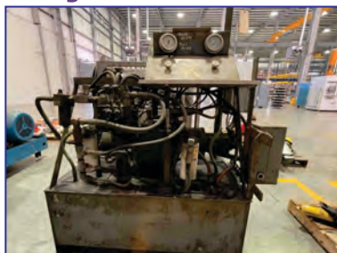
Hydraulic Power Unit, Model K2424CRR, with a 20 hp motor
