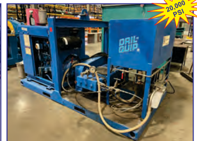
Reliable Pump Inc. Model RD120DS, max. pressure 20,000 psi, 85 hp
