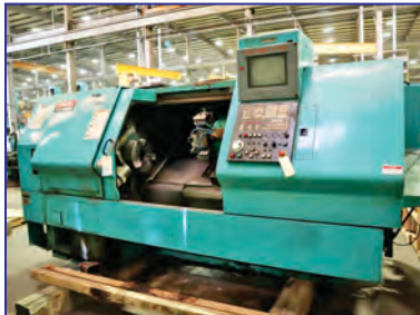
Mazak Quick Turn 25L CNC Lathe, 20.1" swing over bed, 15.76" over slide, 12.6" max. turning dia., 48" max. length, 36 - 3600 rpm, 25 hp, Mazatrol CNC
