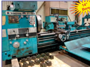
Vanguard S1-262A Hollow Spindle Lathe with 31" 4-Jaw Chuck, 14" bore, 35" swing, 24" over slide, 7 - 305 rpm, 25 hp, threading
