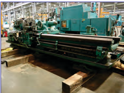
32" x 90" Axelson Engine Lathe with 24" 4-Jaw Chuck
