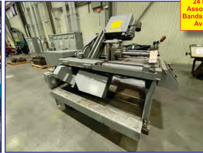
Hem 100LM-2 Tilt Frame Vertical Bandsaw, 18" x 22" cap. at 90 deg., L/R tilt, 65 - 300 fpm, 5 hp
