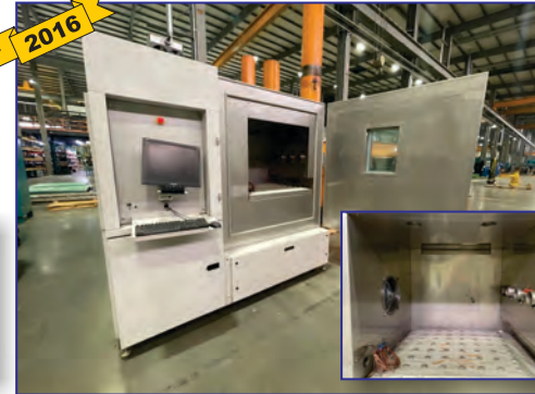
2016 Thermotron Model AST-18 Vibration Thermal Screening Chamber, new 2016, HALT/HASS cap., 50 Grms max. accel., 24" x 24" table, 300 lb. load, -100 to +200 deg. C temp. range, >50 deg. C/min. temp. rate change, 3 linear/3 rotational axes excited
