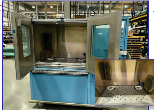
Screening Systems, Inc. Model QRS-410T Vibration Thermal Screening Chamber, HALT/HASS cap., 35 Grms max. accel., 26" x 30" table, 250 lb. load, -60 to +150 deg. C temp. range, 30 - 50 deg. C/min. temp. rate change, SSC-2000 controller, on casters
