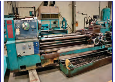
Kingston Heavy Duty 34 Lathe Model HR-2000, 34" swing over bed, 25-1/8" over slide, 80" centers, 8 - 800 rpm, 20 hp, threading, tool post, tailstock
