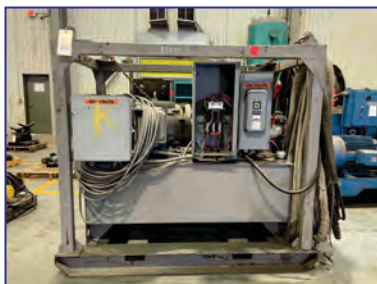
Hydraulic Power Unit with a 40 hp Viking Thor High Efficiency AC motor
