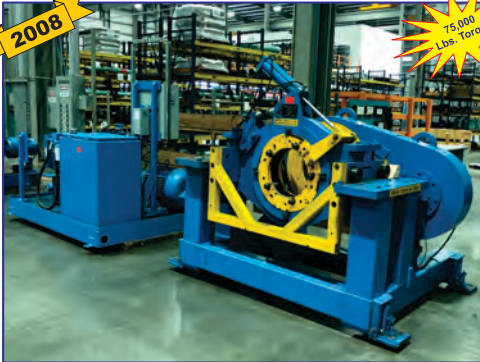
2008 Peck-O-Matic Model 821 Bucking Machine, new 2008, 2-3/8" - 17" O.D. range, 2-3/8" - 16" pipe size range, 4,000 - 75,000 ft.-lbs. torque, 10 rpm (low gear), 20 rpm (high gear)
