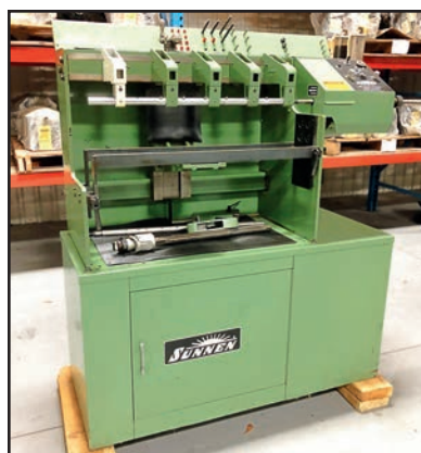
SUNNEN CB-24000K LINE BORING MACHINE
