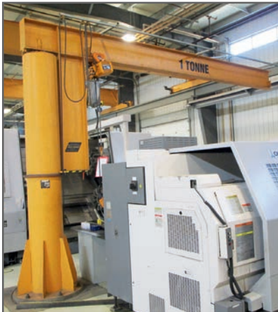
TEKO 1-TON FREE STANDING JIB CRANE
