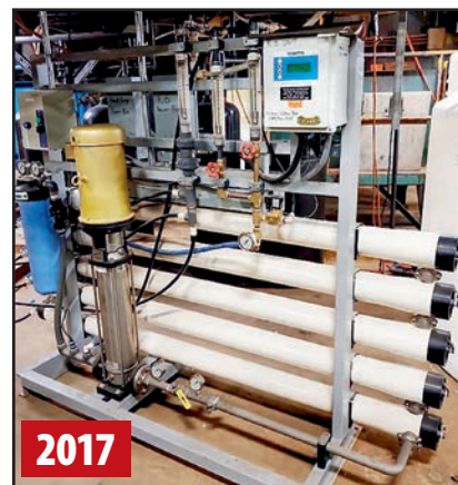
2017 WATTS WATER TECH R24 RO SYSTEM
