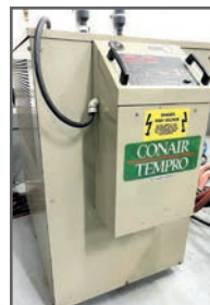
CONAIR TEMPRO MPA-3 PORTABLE CHILLER
