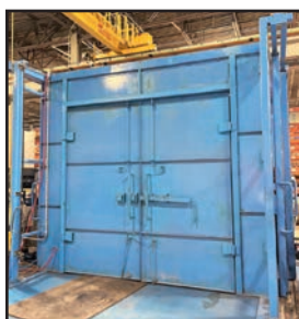
144" X 176" X 144" REINFORCED TEST BOOTH
