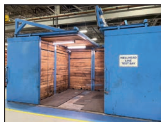
144" X 144" X 120" HIGH REINFORCED TEST BOOTH
