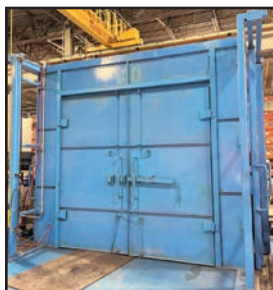
144" X 176" X 144" REINFORCED TEST BOOTH
