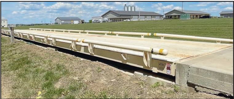
CARDINAL 10080-EPR 80' X 200,000 LB ABOVE GROUND TRUCK SCALE
