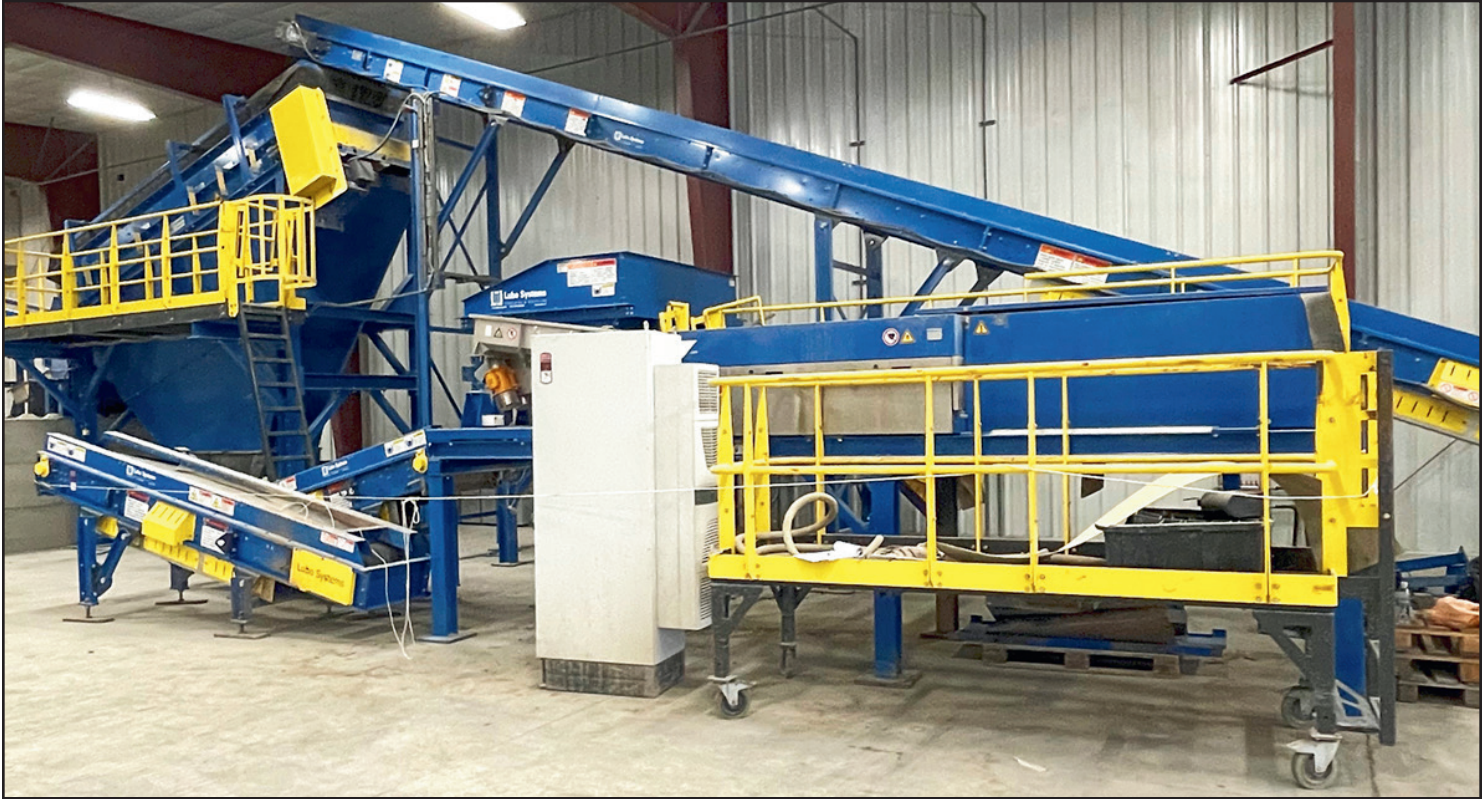
VDL SYSTEMS SPECIAL BUILT METAL RECOVERY EDDY CURRENT SEPARATION LINE
