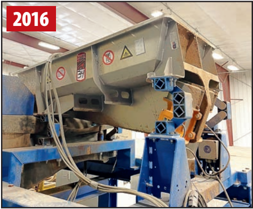
2016 VDL TR84824-01 DIRECTLY DRIVEN SHAKER
