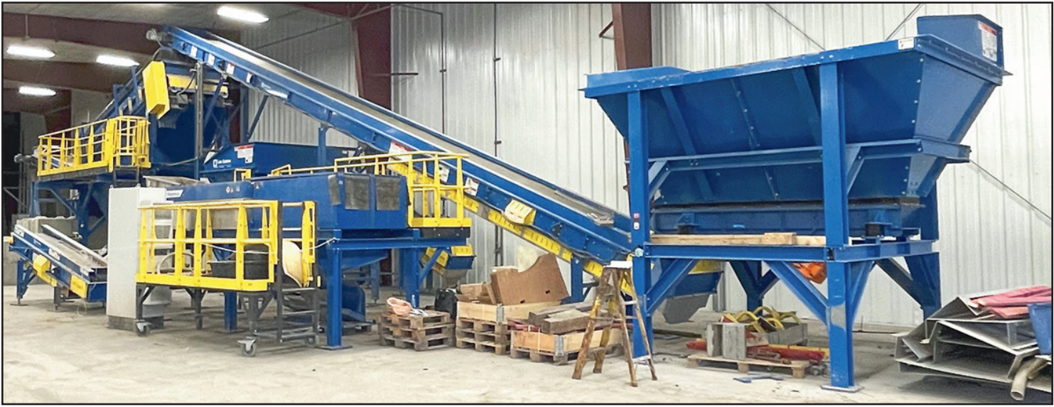
VDL SYSTEMS SPECIAL BUILT METAL RECOVERY SHAKER SEPARATION LINE
