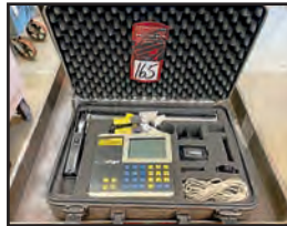
PRUFTECHNIK PT ALIGN ALI2.050 ALIGNMENT SYSTEM
