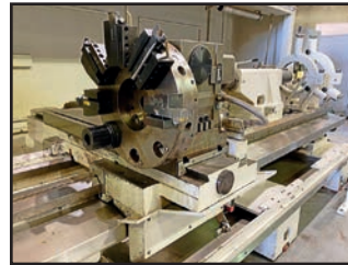
POREBA PNA-80/BARUFFALDI 8-POSITION TURRET, TAILSTOCK AND STEADY RESTS
