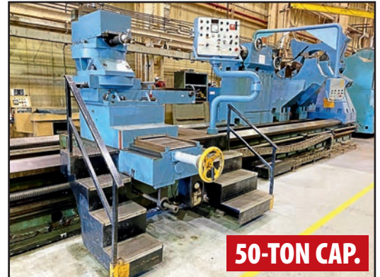
GIANA GFP-24 129" X 421" CARRIAGE, STEADY RESTS AND TAILSTOCK
