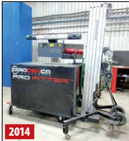
VIRTEK LPS-7H 3D LASER PROJECTOR
