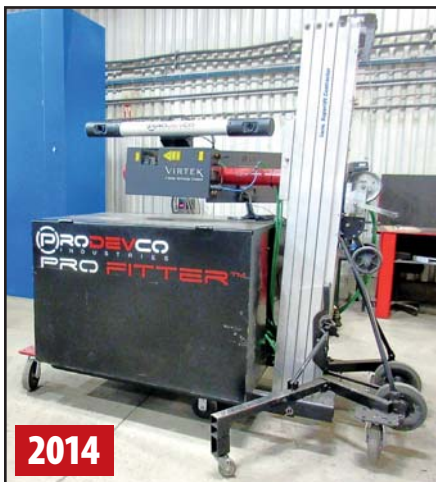
VIRTEK LPS-7H 3D LASER PROJECTOR
