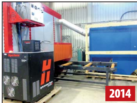
PCR 42-PLASMA AND FUME FILTER
