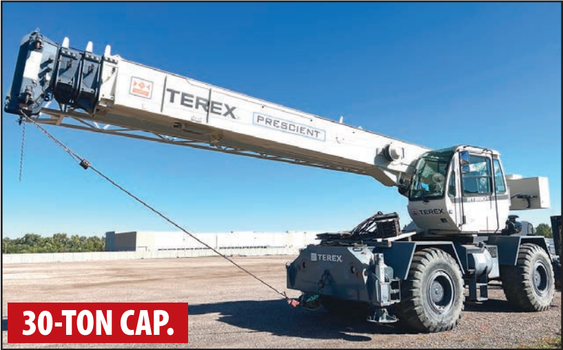
TEREX TR230-1 30-TON MOBILE CRANE
