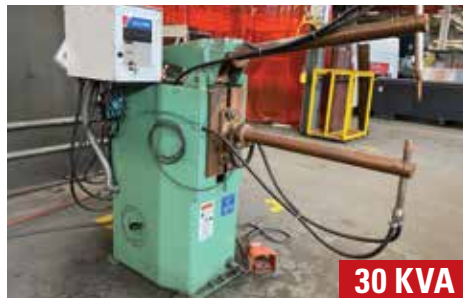
30 KVA FEDERAL RA2-30-30 SPOT WELDER
