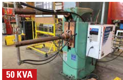
50 KVA FEDERAL RA2-30-50 SPOT WELDER
