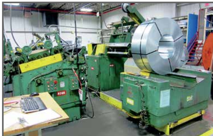
ROWE 30" X .150" X 10,000 LB SERVO COIL FEED SYSTEM
