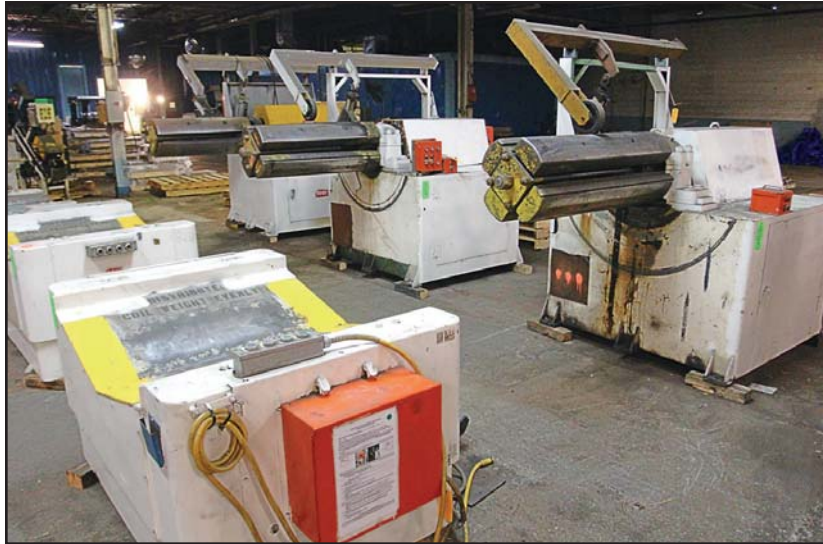
VIEW OF COIL REELS AND BUGGIES
