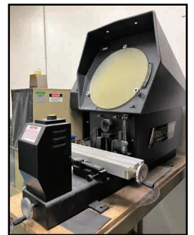
SUBURBAN TOOL MV-14 OPTICAL COMPARATOR
