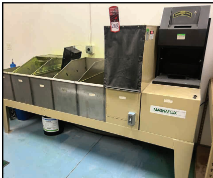
MAGNAFLUX ZYGLO ZD-37 FLUORESCENT PENETRANT INSPECTION SYSTEM
