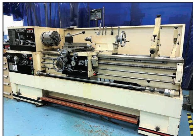
JET GH-1660ZX GAP BED ENGINE LATHE
