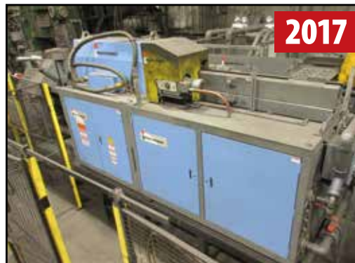
INDUCTOHEAT INDUCTOFORGE 250 KW INDUCTION BILLET HEATER
