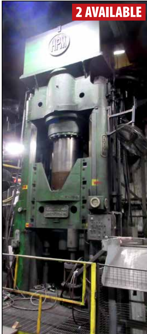
HPM 1000 TON HYDRAULIC HOT FORGING PRESS
