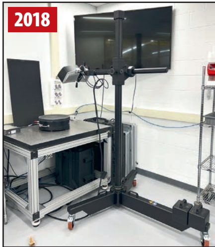
ZEISS COMET 6 BLUE-LED 3D SCANNING SYSTEM
