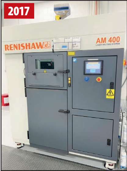
RENISHAW AM400M 400W SINGLE LASER MELTING 3D PRINTER
