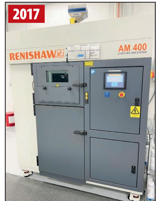
RENISHAW AM400M 400W SINGLE LASER MELTING 3D PRINTER
