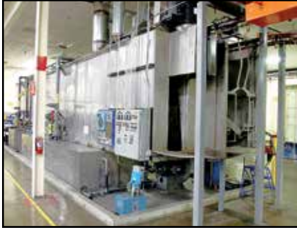
TELLKAMP SYSTEMS 4-STAGE STAINLESS STEEL WASHER
