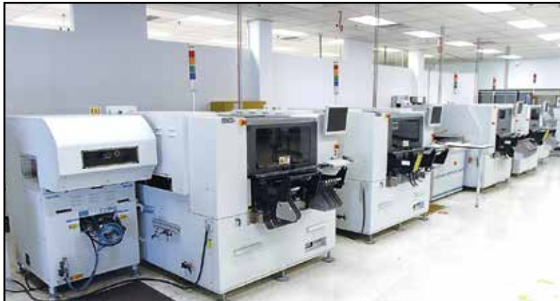
UNIVERSAL ADVANTIS TURN KEY SURFACE MOUNT LINE
