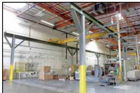
AMERICAN MONORAIL FREE-STANDING BRIDGE CRANE SYSTEM
