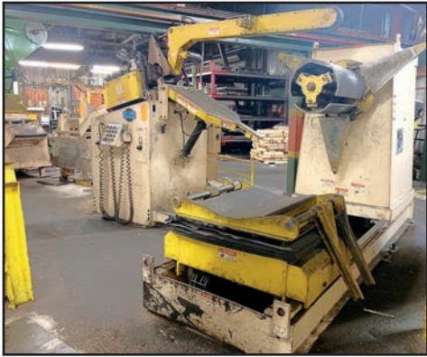
COE COIL LINE (WEAN UNITED SC2-300-72-36 FEED LINE)
