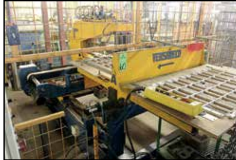
125 KVA CLIFFORD VERSAWELD WELDING CELL
