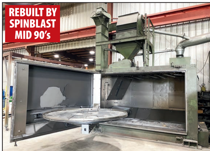
WHEELABRATOR 96" SWING TABLE SHOT BLAST SYSTEM
