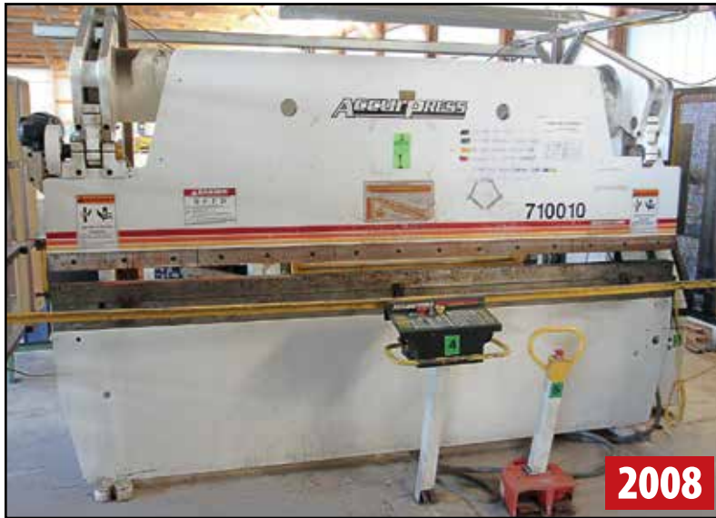
ACCURPRESS 710010 CNC PRESS BRAKE
