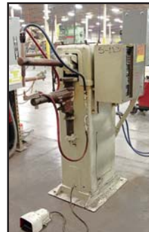
ACMA 3-3-75 75 KVA SPOT WELDER
