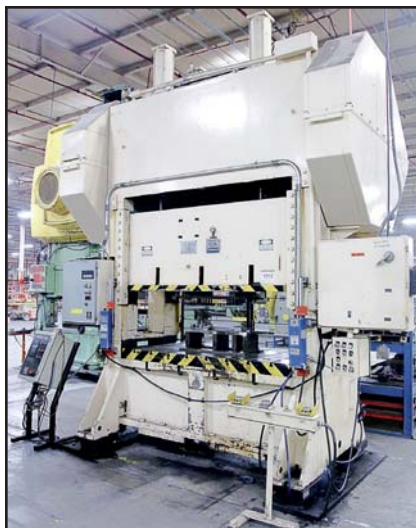
FEDERAL S2-150 150-TON STRAIGHT-SIDE PRESS
