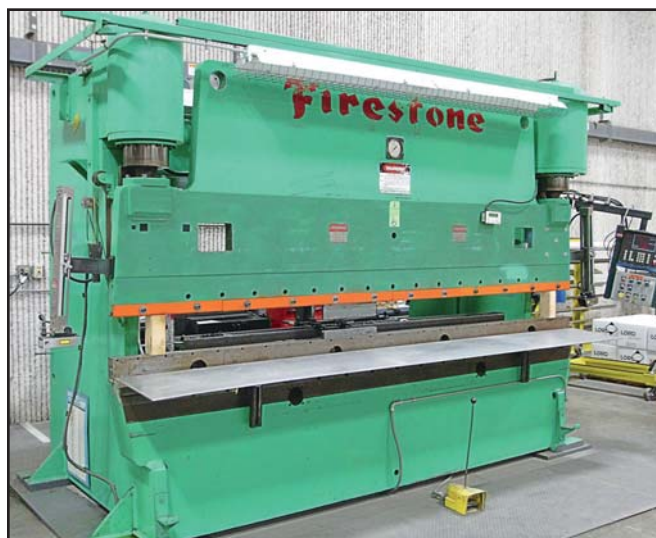
230-TON NIAGARA HD-230-10-12 HYDRAULIC PRESS BRAKE
