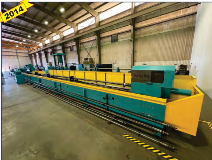
Ohio Tool Works (OTW) 42' Horizontal Hone, 42' Stroke, 1.5" - 20.25" I.D., CNC Control
