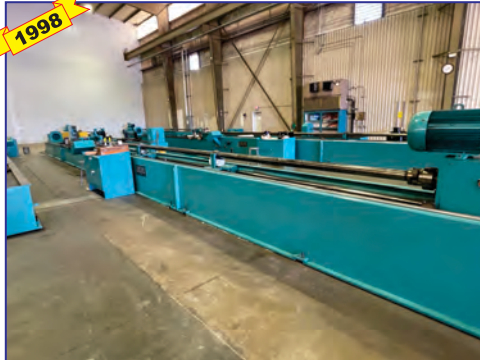
Century Machine 26' Horizontal Hone, 1.5" - 14" I.D. range, 19" max. O.D., 20 HP motor, cycle control, 2 mandrel supports, 2 workpiece clamps, 15 HP fluid pump, paper coolant filtration
