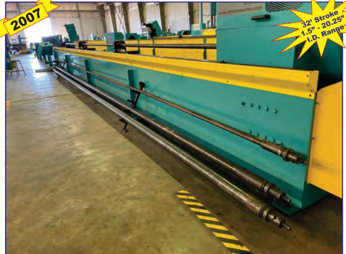
Ohio Tool Works 32' 11" Horizontal Hone, 1.5" - 20.25" I.D. range, 26" max. O.D., 250 rpm, 45 HP motor, touch screen control, 3 mandrel supports, 2 work piece clamps, coolant
