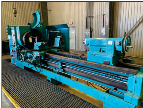
30' x 120" Mazak Model 30 Oil Country Lathe with 12.5" bore, 5 - 300 rpm, 20 HP, 24" front/rear 4-jaw chucks, tool post, taper attach., tailstock, inch/metric threading, coolant
