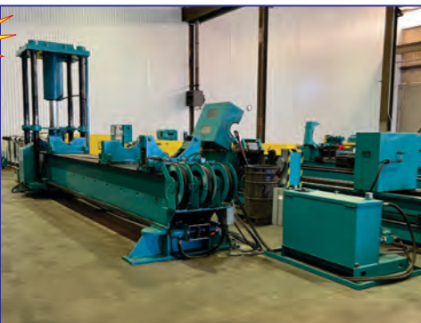
500 Ton Scotia Straightening Press, 26' Bed, 25" Max. O.D.
