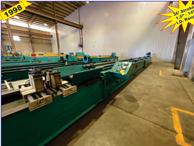
Century Machine 36' Horizontal Hone, 1.5" - 14" I.D. range, 19" max. O.D., 20 HP motor, 3 mandrel supports, 2 work piece clamps, 15 HP fluid Pump, paper coolant filtration
