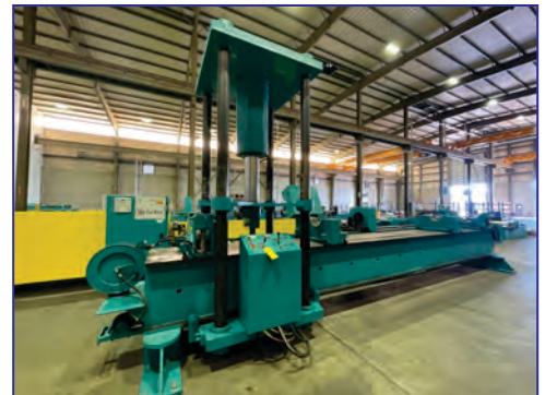
Scotia Drilling Technologies 500 Ton Straightening Press, 26' bed, 24' gantry trvl, 25" max. O.D., 24" cyl. stroke, 30 HP hyd. system, rot. devices, large/small anvils, control console
