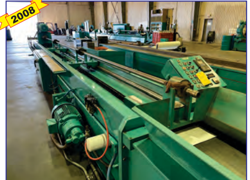
Century Machine 22' Horizontal Hone, 1.5" - 14" I.D. range, 19" max. O.D., 20 HP motor, programmable controller, 2 mandrel supports, 2 workpiece clamps, 15 HP fluid pump, coolant
