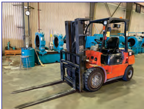
6600 Lb. Dalian Model CPCD30 Forklift, 6600 lb. cap., 20" load center, 50 HP diesel motor, side-shift, 66,393 hours on meter
