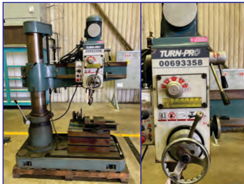
3' 8" Turn-Pro Model RD-900 Radial Arm Drill, 36" arm, 8" dia. col., 6 spindle speeds (88 - 1500 rpm), 2 HP spindle motor, 1 HP feed motor, 3 feeds (0.002, 0.0036, 0.006 ipr), T-slot table
