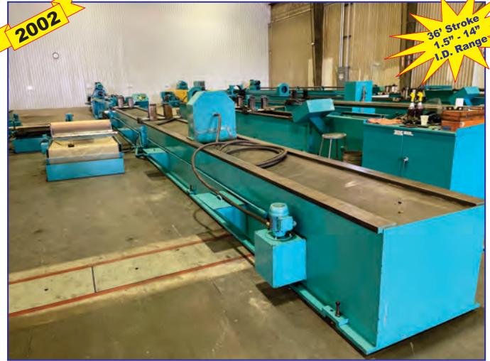
Century Machine 36' Horizontal Hone, 1.5" - 14" I.D. range, 19" max. O.D., 20 HP motor, programmable controller, 3 mandrel supports, 2 work piece clamps, coolant
