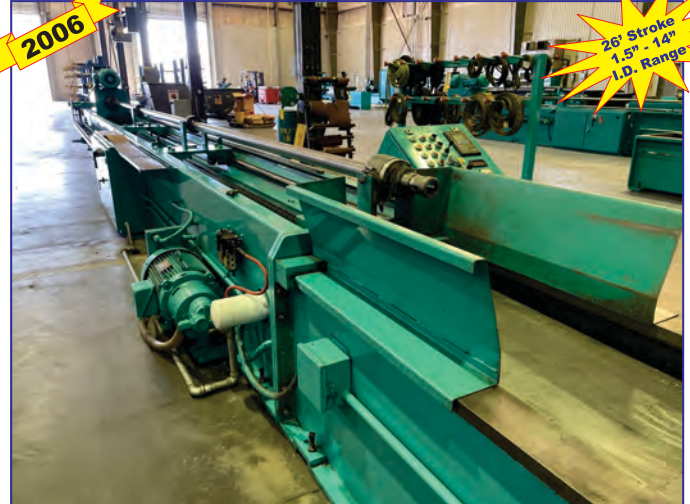
Century Machine 26' Horizontal Hone, 1.5" - 14" I.D. range, 19" max. O.D., 20 HP motor, programmable controller, 2 mandrel supports, 2 work piece clamps, coolant
