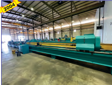
Sunnen 25' Horizontal Hone, 1.5" - 14" I.D. range, 26" max. O.D., 20 HP motor, touch screen control, 2 workpiece clamps, paper coolant filtration
