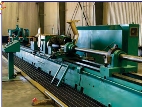
Scotia Drilling Technologies 15' Boring Machine, 15.5' stroke, 3.16" - 10.03" I.D. range, 11.875" max. O.D., 12.5" thru hole, 24" front/rear 4-jaw chucks, 100 HP, boring bars, steadies, coolant
