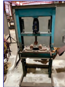
20 Ton Press, w/ 20 Ton Lincoln Hydraulic Jack
