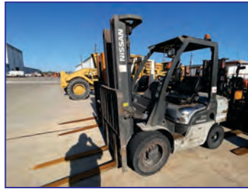
4,800 Lb. Nissan Model MUJL02A28JV Forklift, 187" Lift Height, 24" Load Center, 3F475 Mast, Side Shift, Forks, 6180 Hours on Meter
