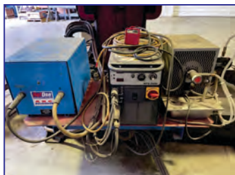
Clad Unit #5: Vanguard LHZ34 Automatic Cladding Machine, Arc Specialties Hot One Solid State Hotwire Power Supply, 118" boom vert. trvl, 175.5" boom hor. trvl, +/-180° col. rot., Esab MTS-3500i MIG Welder, BEST Welds Welding Torch Water Cooler
