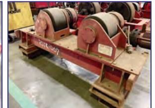
20 Ton Vanguard HGK-20 Turning Rolls
