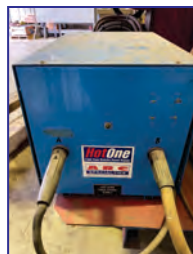
Clad Unit #5: Vanguard LHZ34 Automatic Cladding Machine, Arc Specialties Hot One Solid State Hotwire Power Supply, 118" boom vert. trvl, 175.5" boom hor. trvl, +/-180° col. rot., Esab MTS-3500i MIG Welder, BEST Welds Welding Torch Water Cooler
