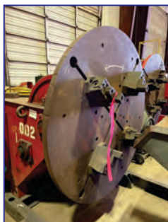
60" Tilt/Turn Welding Positioner w/ 4 HD Jaws
