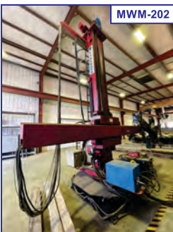
Clad Unit #5: Vanguard LHZ34 Automatic Cladding Machine, Arc Specialties Hot One Solid State Hotwire Power Supply, 118" boom vert. trvl, 175.5" boom hor. trvl, +/-180° col. rot., Esab MTS-3500i MIG Welder, BEST Welds Welding Torch Water Cooler
