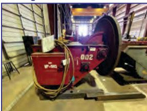
60" Tilt/Turn Welding Positioner
