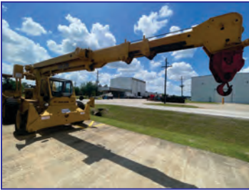
15 Ton Galion Model 150FA Rough Terrain Crane, 18' - 60' Boom Length, 20' Max. Jib Length, 360° Rotation, 70° Max. Elev., 8' 8" Max. Tail Swing, 6' 6.75" Hook Ht. (Boom Horiz.), 121 HP Engine, 26.5 MPH Max. Speed, Outriggers, S/N 10055
