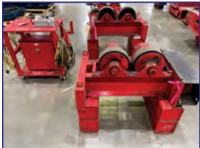
5 Ton Weldwire WWRT 10 Turning Rolls
