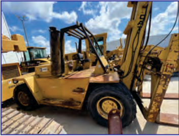
30,000 Lb. Caterpillar Model V300 Heavy Duty Forklift, Type: D, 171" Lift Height, 48" Load Center, 906 Hours on Meter
