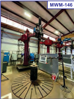
Clad Unit #2: A&N Plant Model RC40X3.75 Cladding Machine (S/N 3163), Arc Specialties Hot One Solid State Hotwire Power Supply (S/N 1216-20436), 100" dia. table, 118" mm boom vert. trvl, 69" boom hor. trvl, 213" overall ht., Esab X Series MTS-3500i Welder (S/N MORJ833003)
