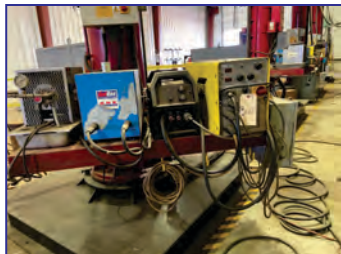
Clad Unit #4: A&N Plant Model RC4X3.75 Cladding Machine (S/N 2558), Arc Specialties Hot One Solid State Hotwire Power Supply (S/N 0999-96006), 100" dia. table, 122" boom vert. trvl, 69" hor. trvl, 218" overall ht., Esab 350 MPI MIG Welder, DC TIG Arc Starter, Best Welds Welding Torch Water Cooler
