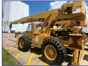
15 Ton Galion Model 150FA Rough Terrain Crane, 18' - 60' Boom Length, 20' Max. Jib Length, 360° Rotation, 70° Max. Elev., 8' 8" Max. Tail Swing, 6' 6.75" Hook Ht. (Boom Horiz.), 121 HP Engine, 26.5 MPH Max. Speed, Outriggers, S/N 10055
