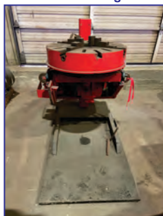
26" Tilt/Turn Positioner w/ 25" 4-Jaw Chuck
